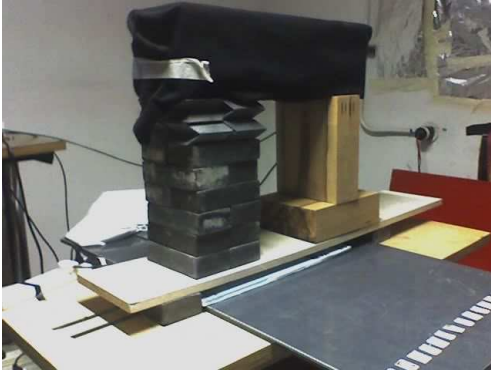
Figure 3. Setup A & B: laboratory conditions and buried detector. lhs : suspended lead column on the module prototype in the laboratory, rhs : service pipe to gain access to the electronics.
